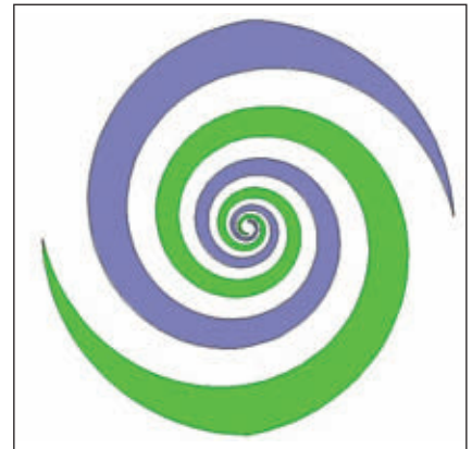
▲ Fig. 4 Typical two-armed equi-angular spiral.
